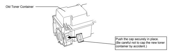
**4.** Dispose of the old toner container in the plastic waste bag supplied in the new toner kit so that toner does not scatter.
